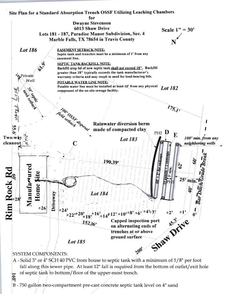
C - 3" or 4" SCH 40 PVC pipe from septic tank to drainfield
