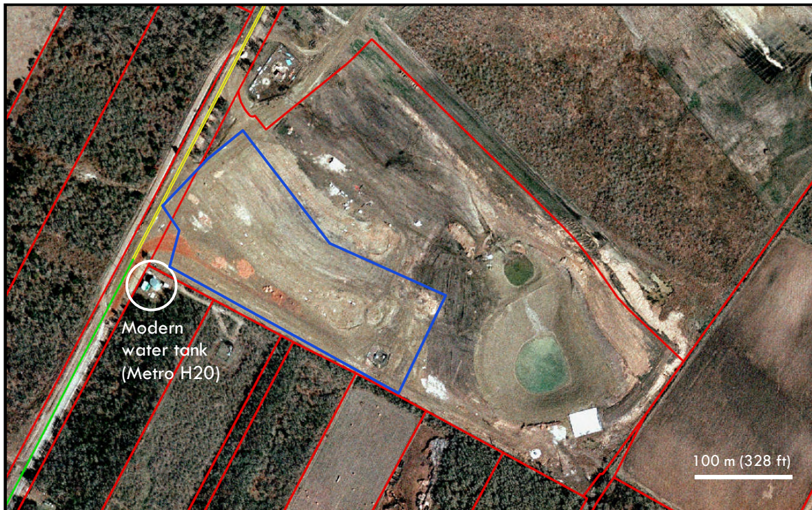
Figure 2. Aerial photograph (2007) with property boundaries marked in red and the project area in blue. The entire project area was bladed and excavated by heavy equipment for utility installation, road construction, and the preparation of residential lots. In addition, various fills were brought in to level the area (visible as contrasting sediment colors). The aboveground water storage tank at the southwest corner of the project area replaced an earlier (although not historic-age) water tank noted on the 1988 USGS map (Manor quad) shown in Figure 1.
